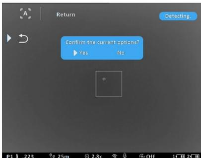
If the message "No bullet holes detected, shoot again" appears, or the small white cross is deviated with the heat signature of projectile impact, it means that the auto zero process has failed, so please follow steps 1 to 5 again.
