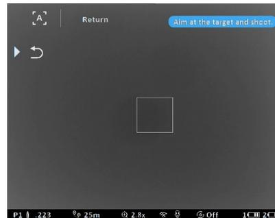
**Step 3:** Aim at the objective or target that is used for zeroing at 25 meters around. Ensure that the 'square reticle' is approximately centered on the target face and then take the shot. The onboard computer will look for the heat signature of the projectile impact on the target face.
