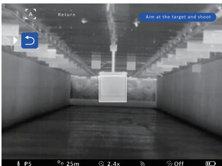
**Step 3:** Aim at the objective or target that is used for zeroing at 25 meters around. Ensure that the 'square reticle' is approximately centered on the target face and then take the shot. The onboard computer will look for the heat signature of the projectile impact on the target face.
