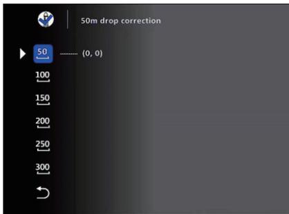
Default value is 0, no correction to the reticle. Select distance, it will enter into the menu below. The message on the lower left corner tells the value in cm for each one click.
