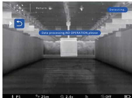
**Step 5:** When message “Confirm the current options?” pops up, click Yes. This confirms that the computer has correctly identified your projectile impact and that the Auto zero process is now complete.
