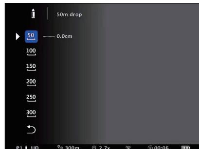
The drop is referred to the zeroing at 0 meter. Up is positive value and Down is negative value.
